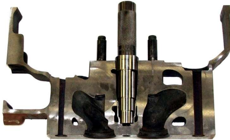
Sleeve Drive-In Tool installing Retaining Ring
