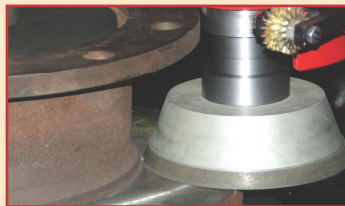
Shown Grinding a HD Truck Rotor
